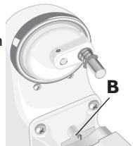
**NOTE:** Flat beater must not strike on bottom or side of bowl when properly adjusted. If beater or wire whip is adjusted too close so that it strikes bottom of bowl, coating may wear off of beaters or wires may wear through on wire whip.
